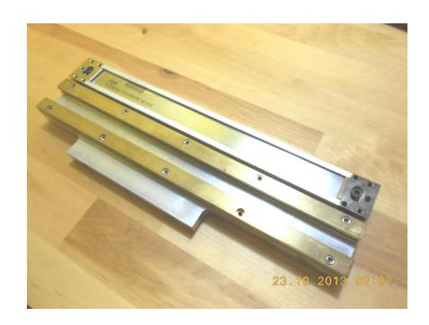
Read head mounting block bolted to sliding rail.
