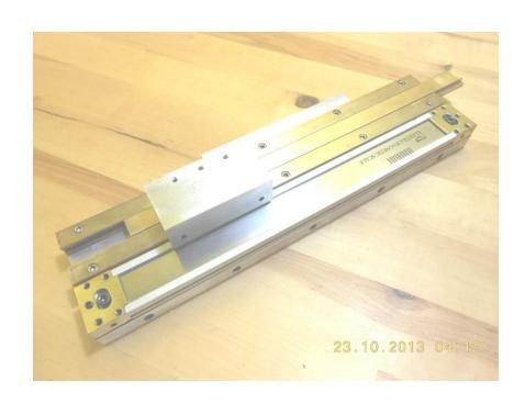
Base plate attached to scale plate.
