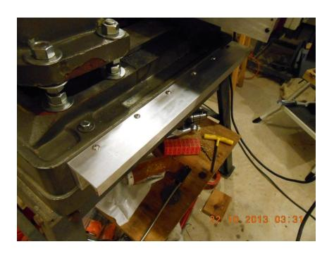
• Read head base plate installed on mill.
