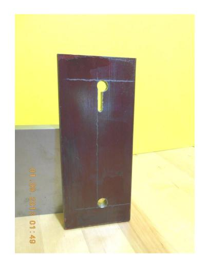
Reciprocating saws will cut 1018 steel but not tool steel.
