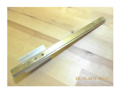
Sliding rail and read head mount installed on scale mounting plate.
