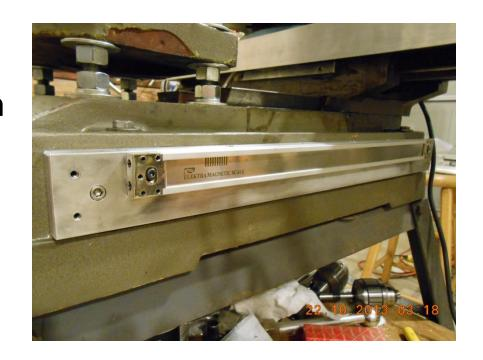
• Y axis swarf shield installed.
