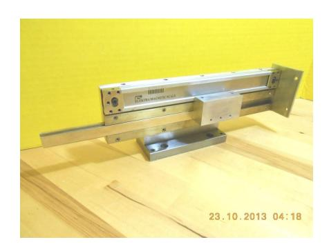
First quill connecting plate attached to sliding rail.
