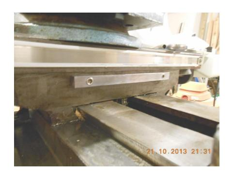
Read head platform attached to base rail with SHCS.
