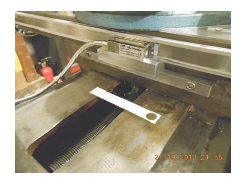
• Swarf shield mounts installed.
