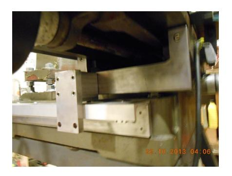
Read head mounting plate installed.
