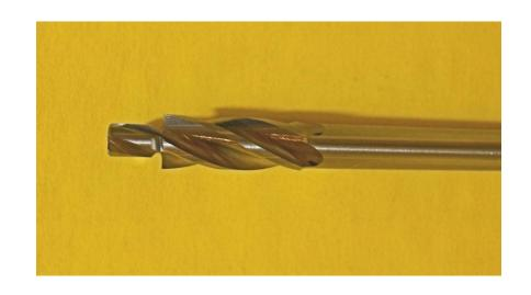
Substituted drill bits for counter bores
