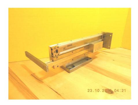
Second quill connecting plate attached to first quill connecting plate.
