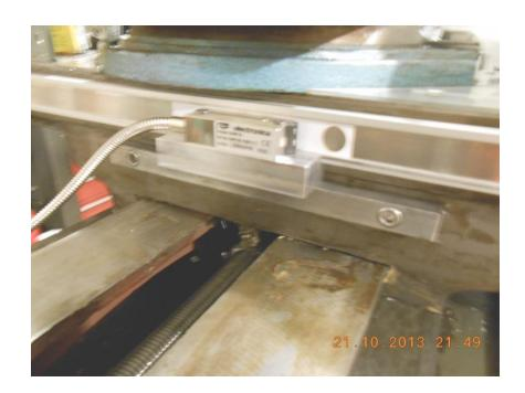
Gauge removal proves read head is not too close to scale.
