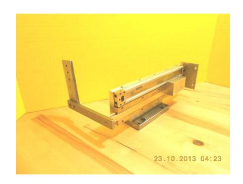
Z axis assembly attached to mill.
