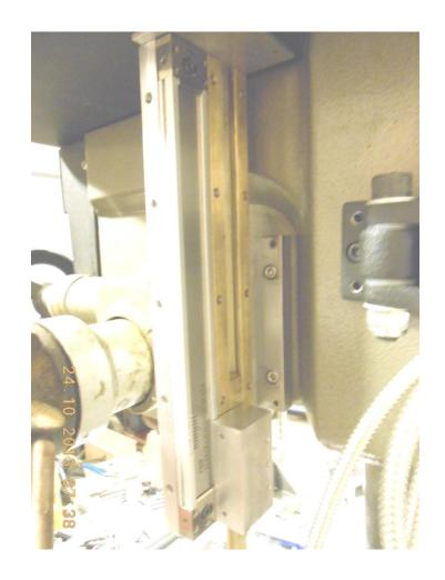
Quill attachment plate bolted to quill and vertical brass slide.
