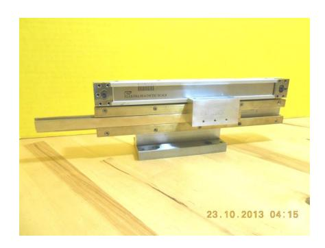
Top side cover installed on scale plate.
