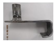
bracket. The bracket is unfinished due to excessive unplanned shrinkage during the bending of a curved section. See photos at left and at right.
